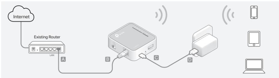
1. Switch the Mode Switch to AP/Rng Ext/Client and connect the hardware from Step A to D.
